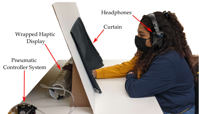
Fig. 3. Experimental Setup. The participants were instructed to sit in the desk right in front of the curtain and put on hearing protection headphones.
