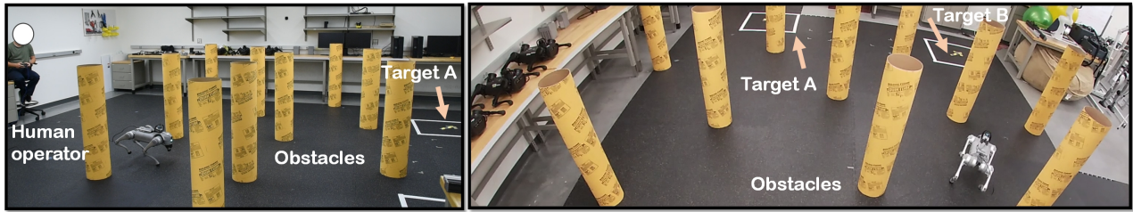
Fig. 1. Side-view and top-view snapshots from one of the 48 human-in-the-loop experiments conducted with 12 participants using the proposed teleoperator-aware CBF-based ANMPC framework. In this trial, the human operator steers the Go2 quadrupedal robot from a designated initial position toward target points, located at the far end of the laboratory, while safely navigating around 10 cylindrical obstacles. The videos are provided in the supplementary file.
