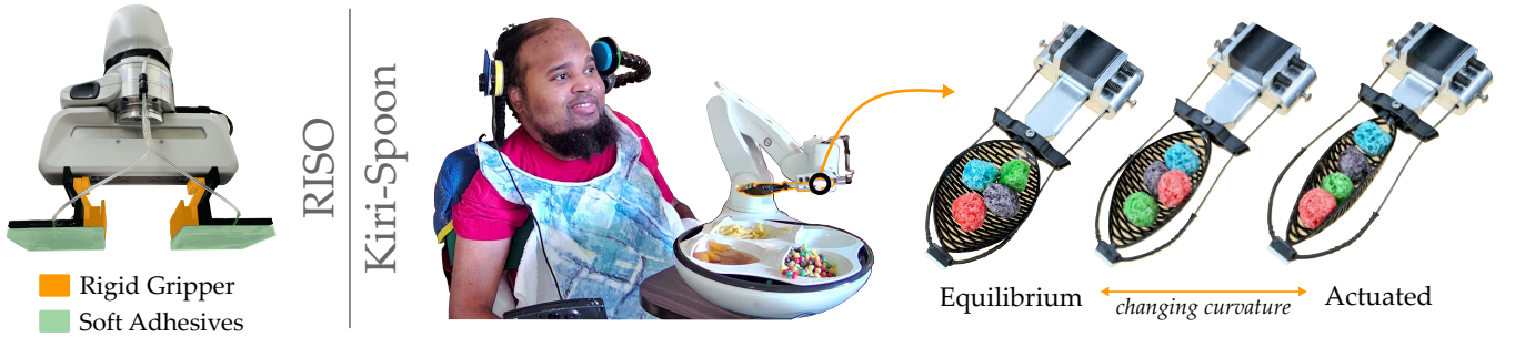
Fig. 5. Applications. (Left) RISO grippers unify traditional rigid end-effectors with a novel class of soft adhesives. When grasping an object, RISOs can either pinch the item between non-deformable fingers or cause the object to stick to soft surfaces. We’ve used RISOs to grasp objects from 2 mg (a piece of lead) to 2 kg (a stack of papers). (Right) The Kiri-Spoon is a soft, shape-changing utensil specifically designed for robot-assisted feeding. Robots using Kiri-Spoons are able to more easily grasp and hold food items, simplifying acquisition and reducing spills.
