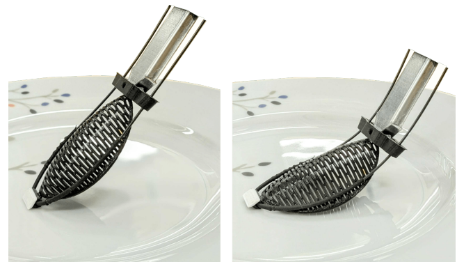
Figure 5. Demonstration of the flexible hoop. This flexibility is not only comfortable for users, but it also enables Kiri-Spoon to bend along the surface of plates and bowls. We leverage this flexibility to deploy Kiri-Spoon like a fork and pinch foods that are directly beneath the kirigami structure.
