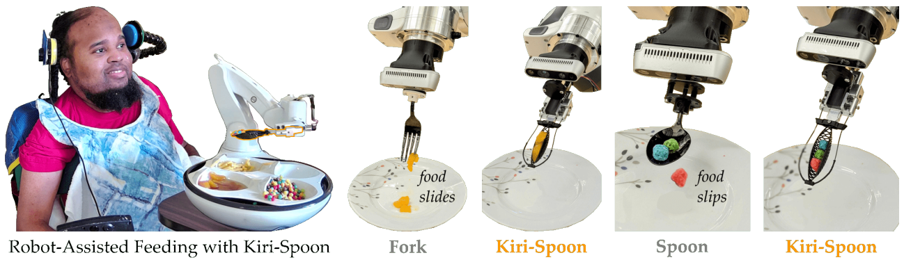
Figure 1. Kiri-Spoon is a spoon-shaped kirigami utensil specifically designed for robot-assisted feeding. (Left) Robot arms equipped with Kiri-Spoon can robustly acquire foods from the plate, safely carry those morsels to the human, and then seamlessly transfer items into the user’s mouth. (Right) It is challenging for robot arms to dexterously manipulate traditional utensils such as forks and spoons. By comparison, Kiri-Spoon makes the robot’s task fundamentally easier by flexibly wrapping around the desired foods. This capability enables Kiri-Spoon to function as a fork (pinching foods) or as a spoon (scooping foods).
