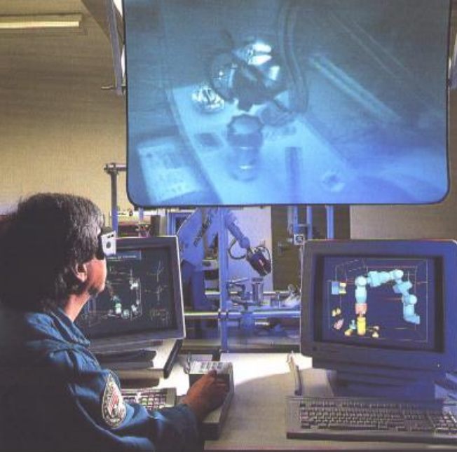
Fig. 2. Robot Technology Experiment (ROTEX) was an early shared autonomy approach, where the robot operated with partial autonomy to complete low-level sensor-based feedback control tasks [18]. Reprinted from [19], with permission from Springer Nature. © Springer Nature 2003.
