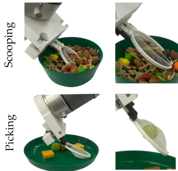
Fig. 1. Human controlling the robot arm and Kiri-Spoon during robot-assisted feeding. The operator relies on the robot arm to pick up and carry food items. Our proposed Kiri-Spoon makes this easier by encapsulating and releasing foods within a soft kirigami structure with adjustable curvature. Using Kiri-Spoon the robot can scoop food from a bowl or pick food off a plate while wrapping around that food firmly to prevent spills.
